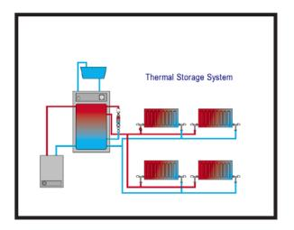
Hot water will be available any time you need it when the system is switched on, summer and winter. But instead of your boiler operation determining when you get hot water and heating, your needs for hot water and heating will determine when your boiler operates.
