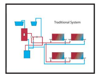
Your central heating still works on a timer which is fitted to your Thermal Store and thermostats control your room temperatures.
