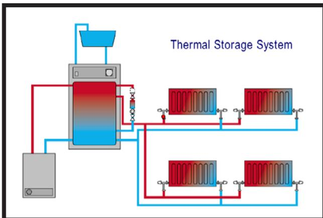
Hot water will be available any time you need it when the system is switched on, summer and winter. But instead of your boiler operation determining when you get hot water and heating, your needs for hot water and heating will determine when your boiler operates.
